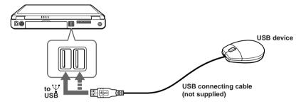
You can use the optional Sony USB mouse PCGA-UMS1 series with this computer. The USB mouse software driver is preinstalled in the computer. Plug the USB mouse into the USB connector, and restart the computer. All necessary drivers will be loaded.
